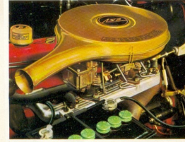
FURY PERFORMANCE of 'X2' comes from twin-carburetors, high-performance camshaft, special inlet/exhaust manifolds, plus new exhaust system. Also features aluminium alloy main bearings.
