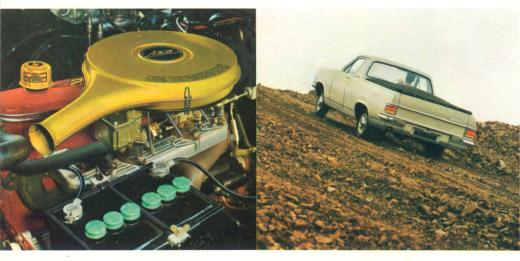
Three Turbo-smooth engines . . . now packing 114, 126 and 145 hp. These powerful increased-horsepower engines are available on both Holden Utility and Panel Van—the standard 114-hp '161' and optional '186' (126-hp) or 'X2' (145-hp). Holden's 'oversquare' engines, with a new, increased compression ratio of 9.2 to 1, are specially designed for Australian conditions. They combine the performance you need in work vehicles with great fuel economy. Holden's exclusive seven-
