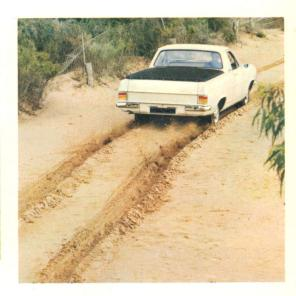
Positive traction rear axle (limited-slip differential): Holden now offers you as an optional extra a limited-slip differential designed to give greater traction on corners, rough ground, in sand or other loose surfaces. So long as one wheel can get a grip, this positive traction axle keeps you going. Ask your Holden Dealer to demonstrate it for you as soon as possible.
