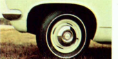
NEW MEDIUM LOW PROFILE TYRES , standard on all models, contribute to Holden's greatly improved ride and road-holding.
