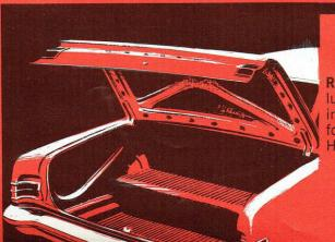
Roomy, easy-to-load boot takes 26 cubic feet of luggage — and its low loading level, ample height inside and vertical spare wheel make it a natural for taxi service. A boot light is now part of the Holden Taxi Package.
