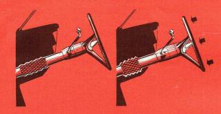
**Energy-absorbing steering column** — pioneered and developed by General Motors — compresses up to 8" under severe impact.
