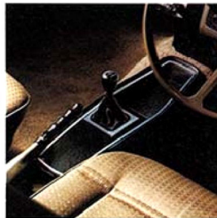
A sporty four-on-the-floor, with synchromesh on every gear, is standard equipment on all models, with console standard on the 'SL'.
