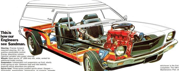
Suspension: Independent coil suspension up front, sturdy 4-leaf spring at rear. Optimum load and ride stability.
