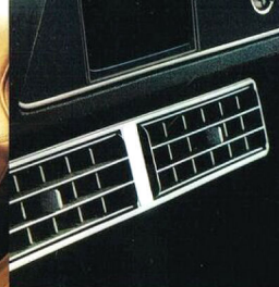
2-speed fan-booster ventilation.
