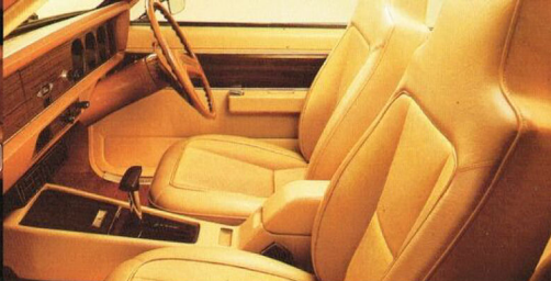
Full foam bucket seats with integral head restraints and a high rise armrest. (T-bar auto. illustrated is an option extra cost.)
