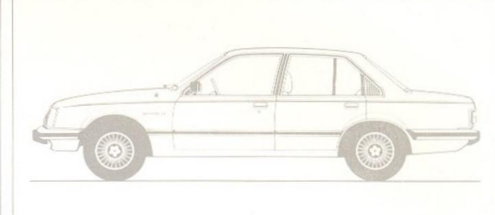
Engine: 2.85 litre six-cylinder. Bore: 88.9mm. x Stroke: 76.2mm. Cubic Capacity: 2838cm<sup>3</sup>. Compression Ratio: 9.2:1. Power Output: 64kW (DIN) @ 4000 rpm. Torque: 198Nm (DIN) @ 2200 rpm. Transmission: 4-speed manual, floor console gearshift. Rear Axle: Salisbury type differential. Rigid axle. Ratio: 3.36:1. Radial Tuned Suspension: Front - MacPherson strut with specially rated coil
