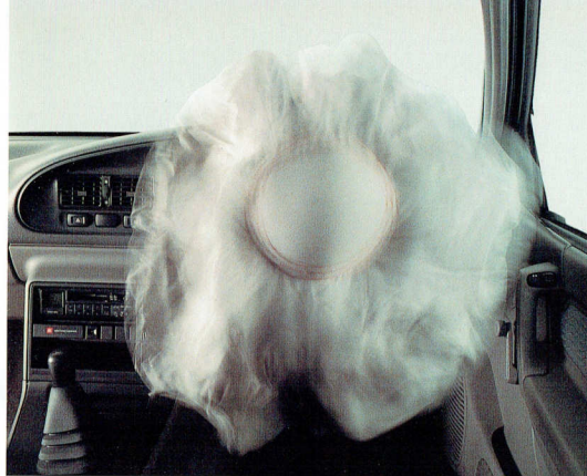
B. 25 Milliseconds. Burst out occurs. The Airbag, housed in the centre of the steering wheel, splits its covering pad in predetermined places and inflates rapidly.
