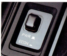
In power mode, the driver now has later upshifts for more engine power.
