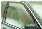
Weathershield for driver and passenger doors keeps rain out and reduces wind in the cabin.
