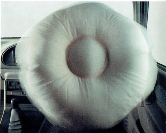
C. 35 Milliseconds. As the Airbag inflates the unique tethers ensure correct positioning.
