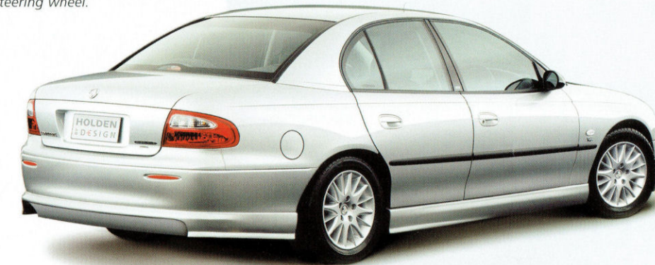
Vehicle fitted with Holden By Design sports body kit and 16" x 7.5" 'T' series alloy wheels.
