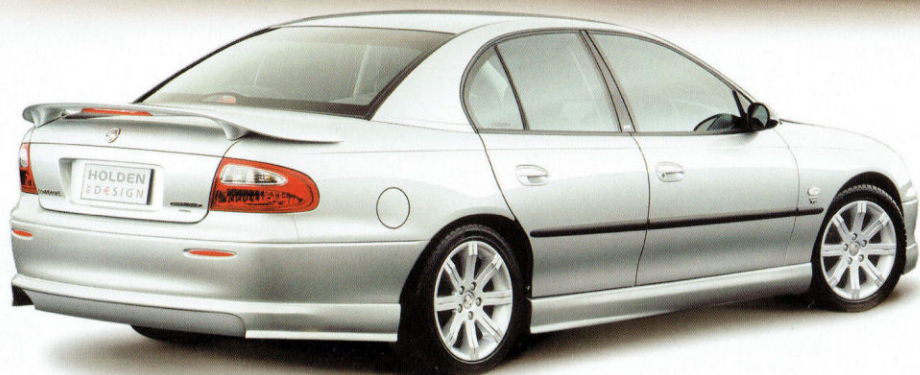
Vehicle fitted with Holden By Design sports body kit, Type 3 sports wing and 17" x 8" 'X' series alloy wheels.
