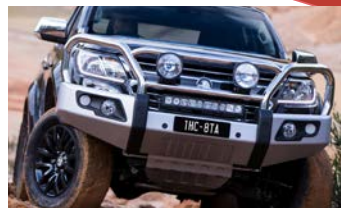
Nullarbor polished steel bull bar with LED light bar (HID driving lights shown not included)
