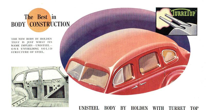
Look at the sectional view above, and you will see that this Unisteel Body by Holden is all steel throughout, just as the name implies. Overhead is the one piece all-steel Turret Top, arched and crowned for the greatest possible strength, and braced with steel cross bows. Underneath is the solid steel floor. Front and side pillars are steel again. The frames of the doors and their panels, all are of steel.
