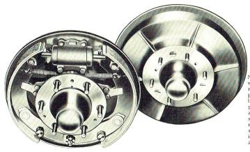
Note the design of the brakes which have self-energizing shoes, reducing the amount of pedal pressure necessary. The brake linings are of extra thickness to give long life, while the shoes are adjustable to take up wear simply by turning two exterior nuts on each brake drum dust shield. The drums are of cast iron ribbed for heat dissipation and to prevent distortion.
