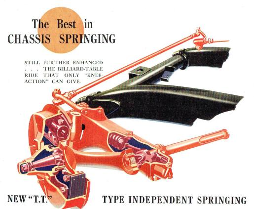
The Vauxhall 25 incorporates a type of Independent Front Wheel Springing with important new features. The system has been called the T.T. type because it embodies a torsion bar and torsion tube and possesses these advantages:
