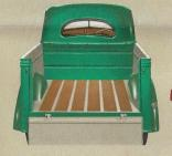
capacity with a hardwood floor laid between the steel longitudinal members. High-grade and practical construction.
