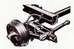
INDEPENDENTLY SPRUNG FRONT WHEELS: The famous Vauxhall patented "torsion-bar-and-tube" independent front wheel springing is used on both Velox and Wyvern. The mechanism, which incorporates sturdy shock absorbers, is designed to give progressively stiffer suspension as the wheels encounter increasingly rough roads. A gliding ride over any type of road.
