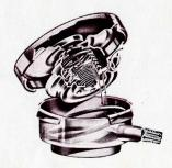
VELOX PRESSURE COOLING: Apart from a larger Fan and radiator than Wyvern, Velox features a welcome innovation in pressure cooling. The cooling system operates at a pressure of 3\frac{3}{4} pounds per sq. in. above normal so raising the boiling point of the water to 223° F. and obviating the necessity of frequent topping up when driving under extreme conditions.
