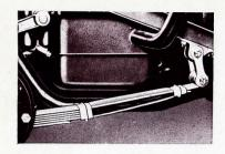
GAITERS ON REAR SPRINGS: A permanent answer to squeaking rear springs is supplied by the use of extended gaiters, or grease sleeves around the rear spring leaves. These neat sleeves are filled with grease and held securely in place by spring collars. They play a big part in giving to Vauxhall its famous shock-free, smooth and eversilent ride
