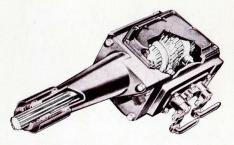
SILENT SYNCHRO-MESH GEARS: The new gear box is designed to transmit the high torque of the Velox engine. The same gear box is used in the Wyvern. It has the famous Vauxhall controlled-type synchro-mesh gears on top and second and it is almost impossible to clash the gears. The extended rear cover allows for a shorter and vibrationless propeller shaft.
