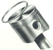
NEW OIL RINGS IMPROVE OIL ECONOMY. Oil scraper rings are now of narrow land type with wider groove, which enables them to "bed down" more quickly and improve oil economy during initial running period. The top compression ring is chromium plated for longer life, less bore wear.
