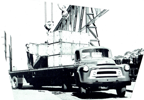
International model AS-162, above, is equipped with an ABD-264 Engine and two-speed rear axle for heavy-duty haulage.
