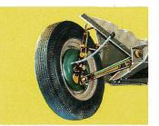
**SUSPENSION:** The independent front suspension is by pre-stressed torsion bars and powerful shock absorbers (56% increased piston area). Rear suspension by semi-elliptic springs
