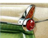
REAR LIGHTS: Set in attractively angled fins, the rear light fittings include tail lights and self-cancelling flashing turn indicators. These direction indicators are also incorporated with the front parking lights.
