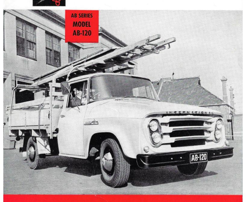
Choose a heavy-duty one-ton truck for your toughest jobs. AB-120 models have full-floating rear axles, 4-speed transmission coupled with the new Gold Diamond engine, for stability and high average speeds on all types of roads.
