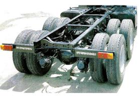
Chassis frame Rugged construction high tensile heat treated frame with Grade 8 flange head bolted construction. For extended durability in harsh Australian driving conditions.
