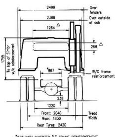
\*879 WITH INVERTED "L" FRAME REINFORCEMENT
