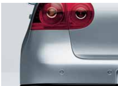
Rear Parking Sensors
