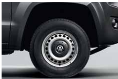
16-inch steel wheels. With 205 R16 C 110/108T tyres.
