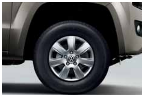
16-inch "Taruma" alloy wheels. With 245/70 R16 111T tyres.
