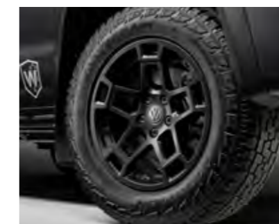
18" x 8.5" forged Alloy Wheels | W580X | With 265/60 R18 Pirelli Scorpion ATR Plus Tyres
