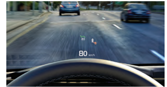
Heads-up display (HUD) 1 lets you keep your eyes on the road by subtly projecting key driving information on the windshield.
