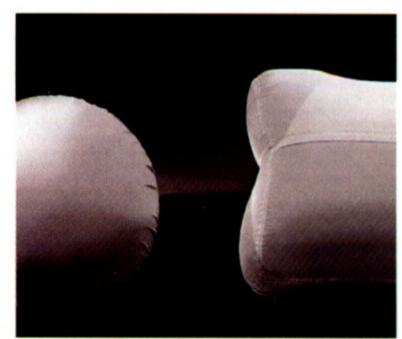
Driver and front-passenger air bags are standard. These air bags have been designed to provide you with enhanced protection when used in conjunction with safety belts. A special note: always wear safety belts, even with
