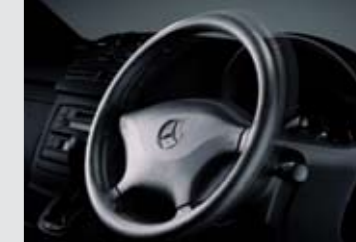
The steering wheel is adjustable for height and reach.
