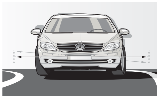
Active Body Control (ABC) The ride height can also be adjusted manually via the COMAND interface when negotiating a particularly poor road surface or when required by the vehicle's load status
