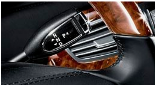
DIRECT SELECT Briefly moving the steering-column selector lever is all it takes to change gear
