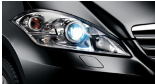
Bi-xenon headlamps/cornering light function for optimum visibility
