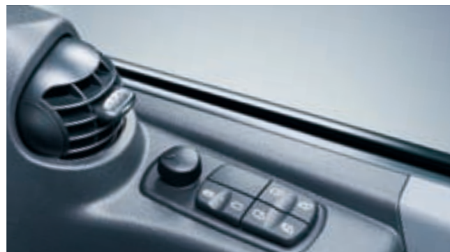
The new door operating panel with easy-to-use function buttons: for adjusting the exterior mirrors on the driver's and co-driver's side, switching the exterior mirror heaters on/off, operating the power windows on the driver's and co-driver's side and – as an option – activating the central locking.
