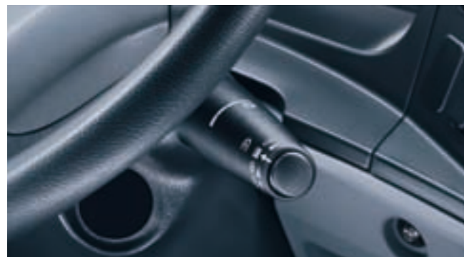
Acceleration and braking: a single control stalk is used to operate the cruise control and engine brake functions.
