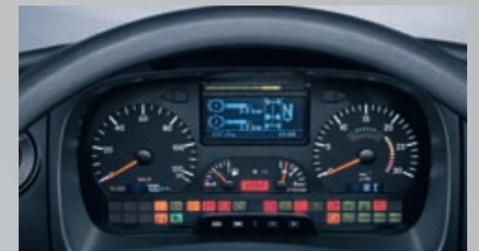
The anti-glare instrument cluster: the function check covers the most important vehicle data and functions and apart from the tyre checks, assists the daily exterior checks of the vehicle carried out by the driver.
