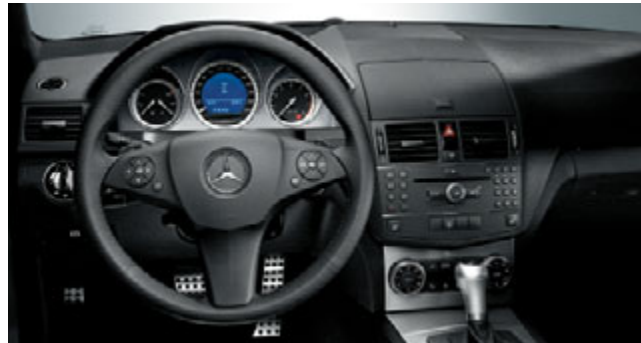
Behind the 3-spoke leather steering wheel are shift paddles for manual gear changes (in conjunction with automatic transmission)
