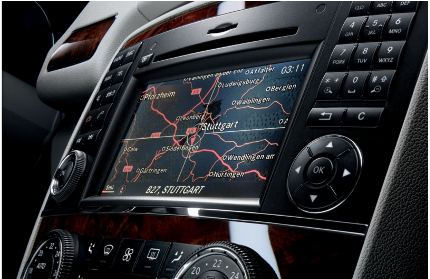
COMAND APS with its clearly legible 6.5-inch colour display
