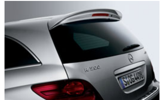
For enhanced aerodynamics: the roof spoiler
