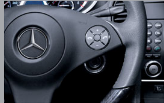
The multifunction buttons give you the option of controlling many of the COMAND APS system's functions directly from the steering wheel
