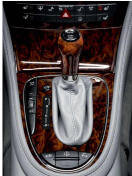
The start/stop button for the optional KEYLESS-GO system is located on the selector lever knob
