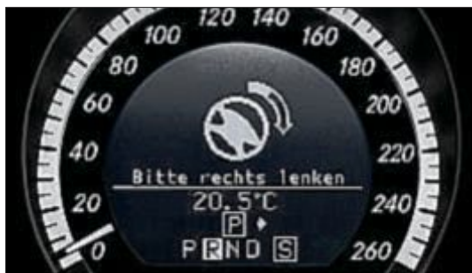
Parking Guidance indicates suitable parking spaces to the driver and provides parking directions
