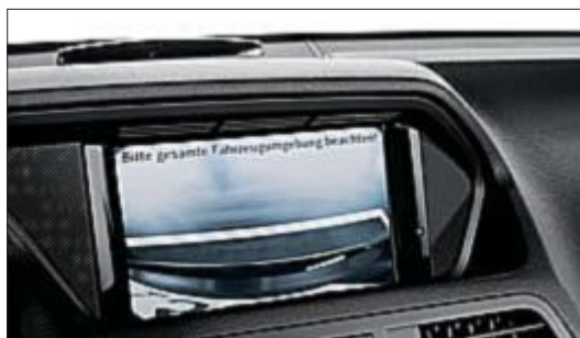
The reversing camera shows the area behind the tail end of the vehicle which is difficult to see
