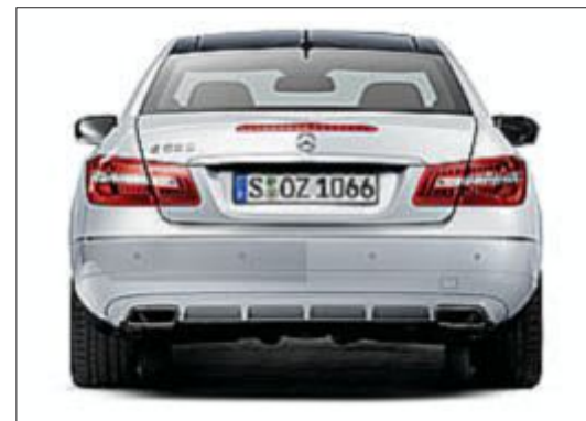
The two-pipe exhaust system with its trapezoidal tailpipes distinguishes the 8-cylinder model
