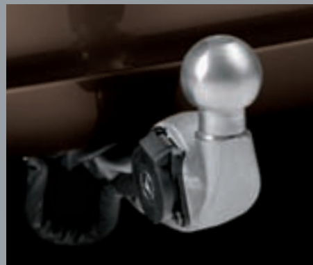
Trailer coupling Fold-away trailer coupling with ball head, control in boot. Drawbar load of 88 kg
