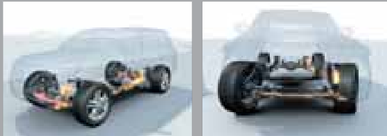
KDSS # significantly reduces body roll when cornering.
