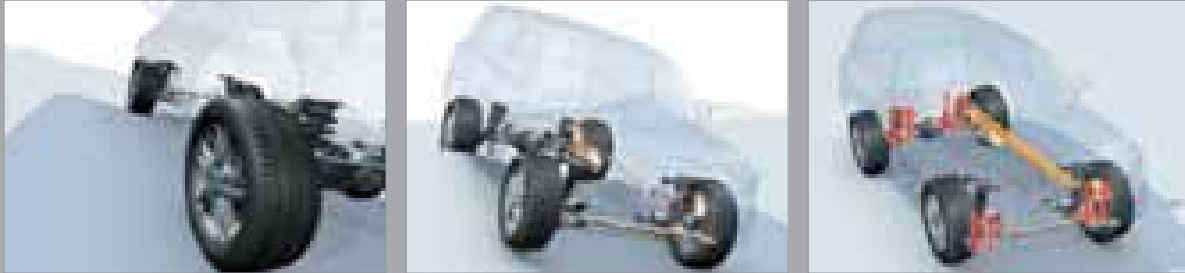
KDSS # enhances wheel articulation in off-road situations for more traction.
