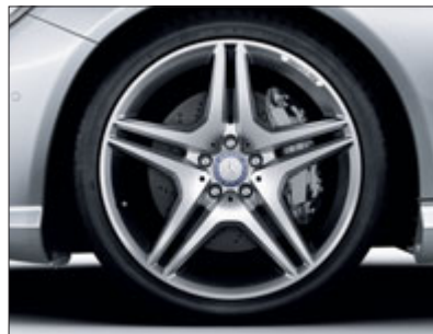
AMG 5-twin-spoke light-alloy wheels with 255/35 R 20 front and 275/35 R 20 rear tyres, 255/35 R 20 tyres all round on 4MATIC models (optional)
