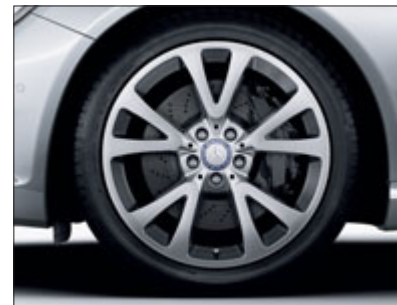
incenio "Nuklida" 5-Y-spoke light-alloy wheels 1 for 255/40 R 19 front and 275/40 R 19 rear tyres, 255/40 R 19 tyres all round on 4MATIC models, titanium silver, high-shine finish (accessory)
