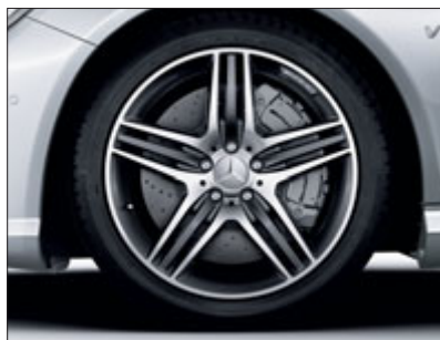
AMG triple-spoke light-alloy wheels with 255/40 R 19 front and 275/40 R 19 rear tyres (standard for CL 63 AMG)
