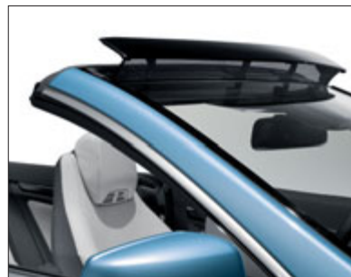
AIRCAP (air deflector module) for the cabriolet
