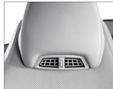
The neck-level heating AIRSCARF for the cabriolet
