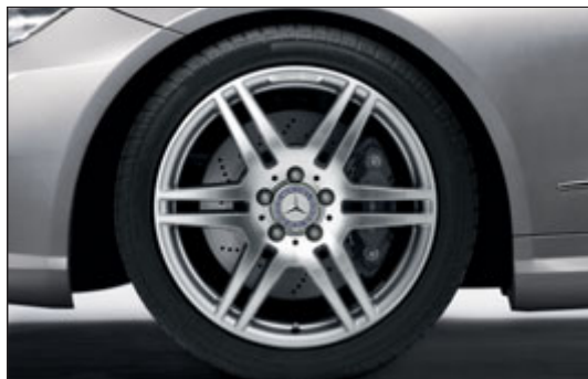
6-twin-spoke AMG light-alloy wheel with 235/40 R 18 front and 255/35 R 18 rear tyres, high-shen (Code 786, part of AMG Sports package)
