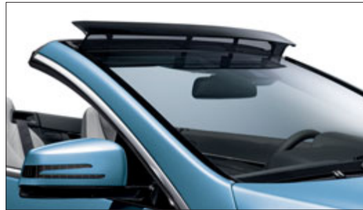
The electric air deflector module on the front of the roof frame is an integral part of AIRCAP
