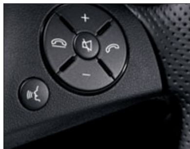
Voice-operated control system LINGUATRONIC with button on steering wheel
