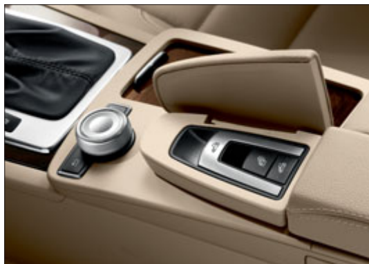
The soft-top operating switch is positioned beneath the handrest for the Controller
