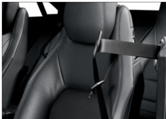
The automatic belt feeder extends the seat belt
