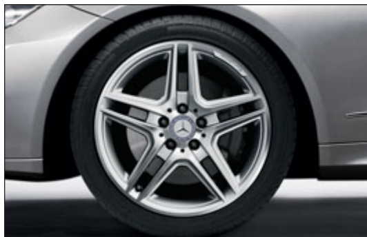
AMG 5-twin-spoke light-alloy wheel with 235/40 R 18 front and 255/35 R 18 rear tyres, high-shen (optional, Code 795)
