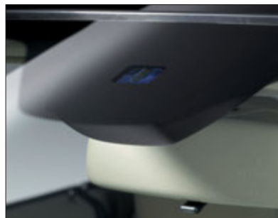
Rain sensor & light sensor for Headlamp Assist
