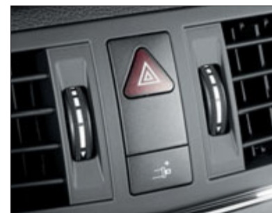
Belt feeder button on the upper dashboard
