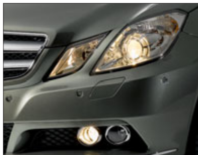
Proj.-beam headlamps, front fog lamps & daytime driving lights
