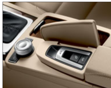
Soft-top operating switch for the cabriolet
