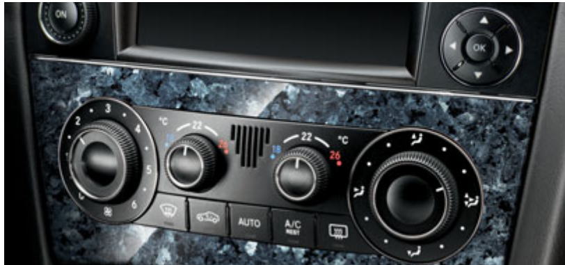
Control panel for air conditioning
