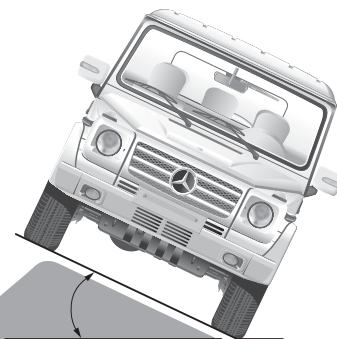
Directionally stable on lateral slopes up to 54%
