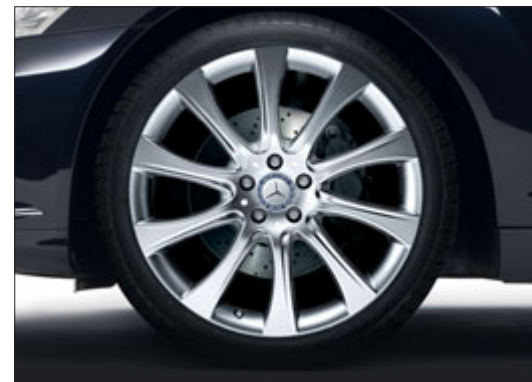
incenio "Alaraph" 10-spoke light-alloy wheel 1 for 255/35 R 20 front and 275/35 R 20 rear tyres (accessory wheel available ex factory)
