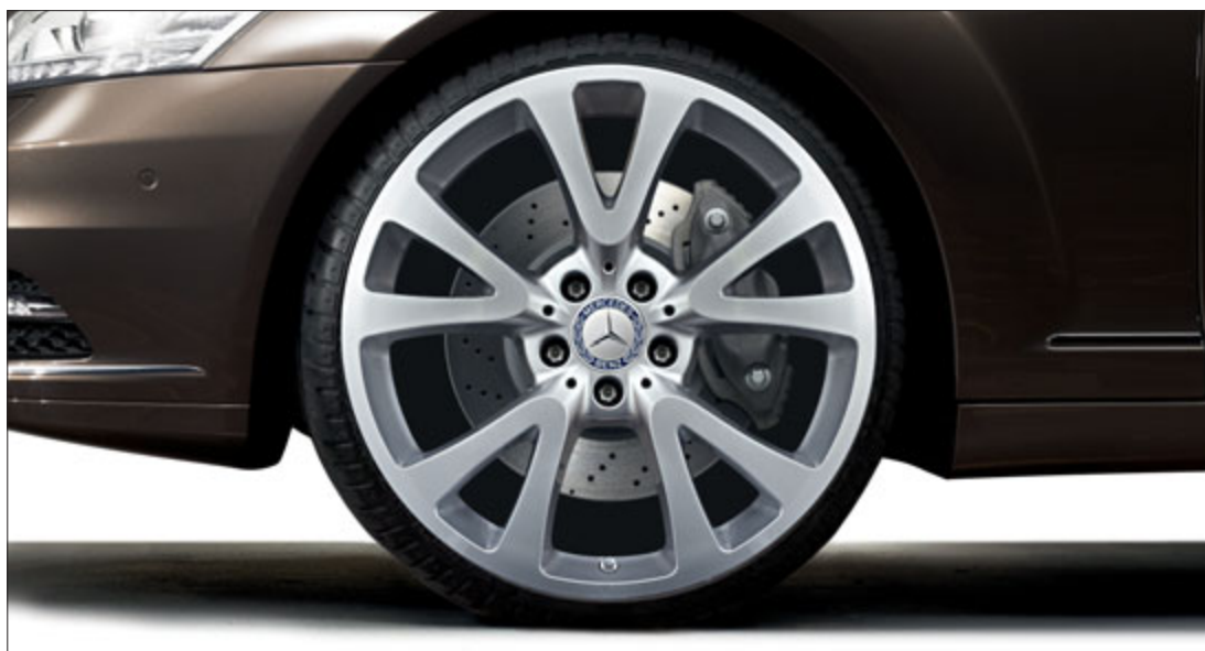
incenico "Nuklida" light-alloy wheel for 255/40 R 19 front and 275/40 R 19 rear tyres, finish in titanium silver, high-shine
