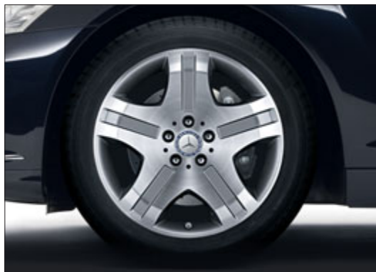
5-spoke light-alloy wheel with 255/45 R 18 front and 275/45 R 18 rear tyres (standard for V12 engine)
