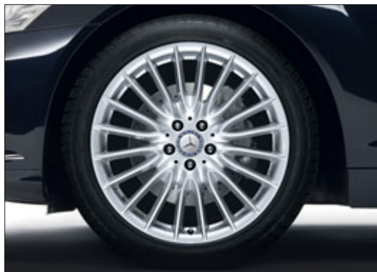
Multi-spoke light-alloy wheel with 255/40 R 19 front and 275/40 R 19 rear tyres (optional extra)
