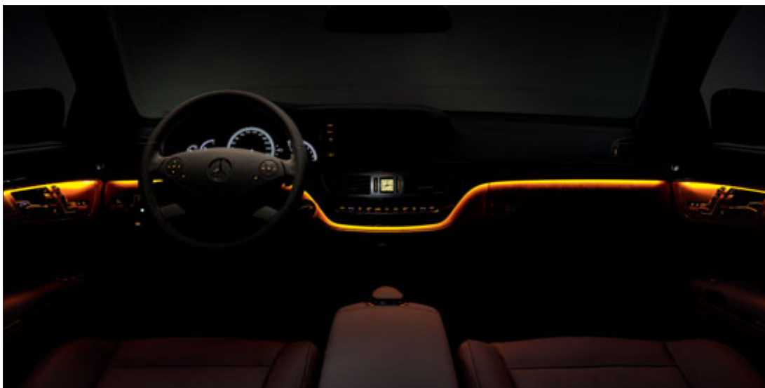
The ambient lighting shines as a narrow band of LEDs along the wood trim, the dashboard and all four doors. These lights are dimmable and can be made to come on in one of three different colours
