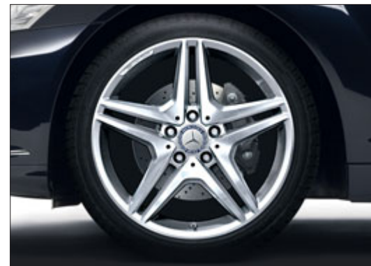
AMG 5-twin-spoke light-alloy wheel with 255/35 R 20 front and 275/35 R 20 rear tyres (optional extra)
