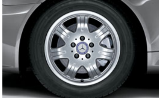
7-spoke light-alloy wheel with 205 / 55 R 16 tyres (standard for SLK 200 KOMPRESSOR)
