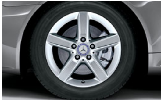
5-spoke light-alloy wheel with 205 / 55 R 16 tyres at the front and 225 / 50 R 16 at the rear (standard for SLK 300, optional for SLK 200 KOMPRESSOR)
