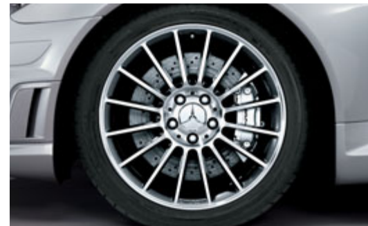
AMG multi-spoke light-alloy wheel in high-shine, titanium-grey-painted finish, with 225/40 R 18 tyres at the front and 245/35 R 18 at the rear (standard for SLK 55 AMG)
