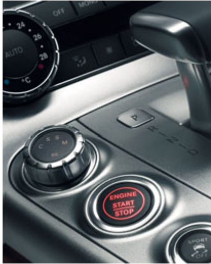
The AMG DRIVE UNIT with E-SELECT lever and KEYLESS GO start function
