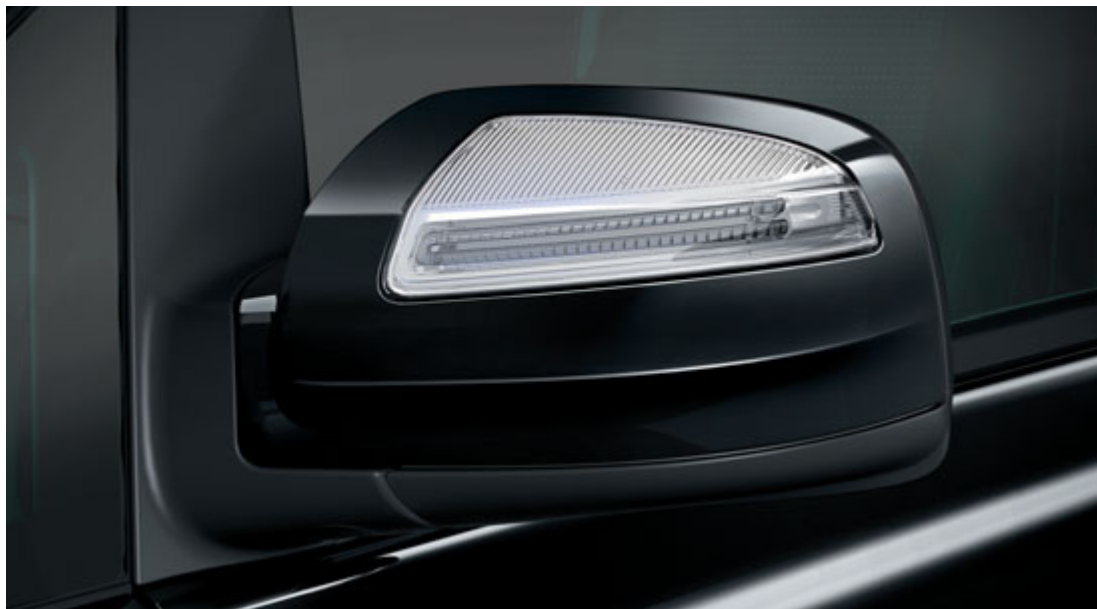
Exterior mirrors with enlarged field of vision and integral indicators, electrically adjustable
