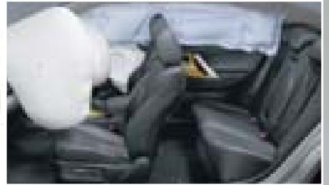
Driver and front passenger, front side and full length curtain SRS airbags
