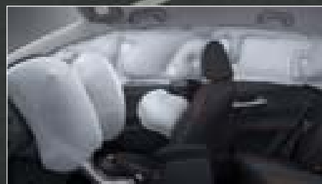
Dual front SRS airbags, front seat mounted side SRS airbags, driver's knee SRS airbag and side curtain shield SRS airbags*
