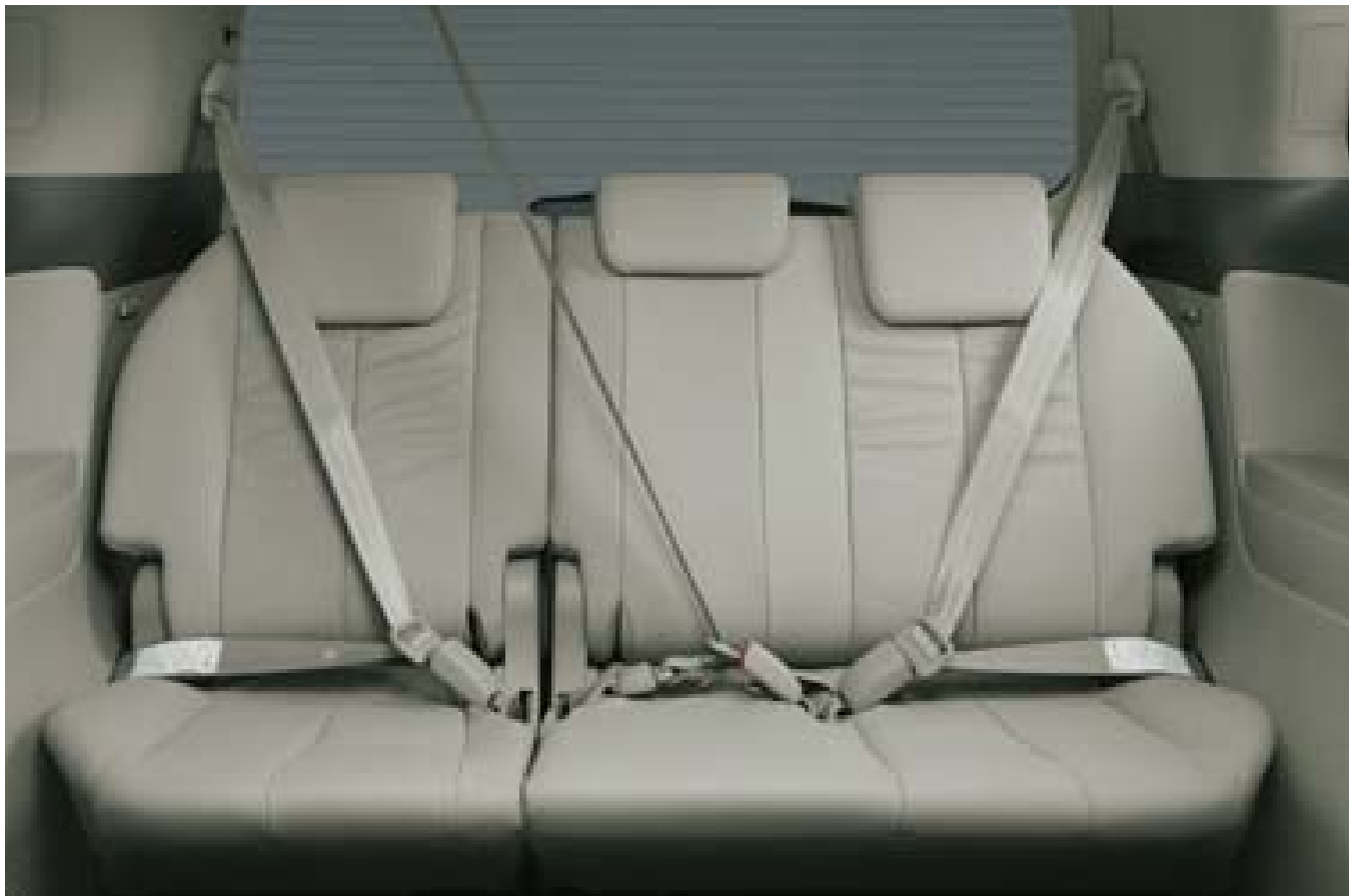
Third row seats with 3-point seatbelts fitted with Emergency Locking Retractors (ELR). Ultima model shown.
