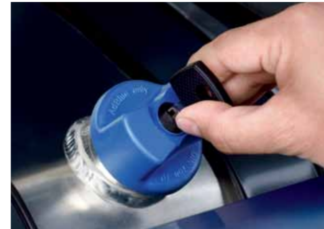
AdBlue is odourless, non-toxic and simple to refill. SCR diesel technology blends AdBlue with the exhaust flow to reduce the nitrogen oxides in the catalytic converter.
