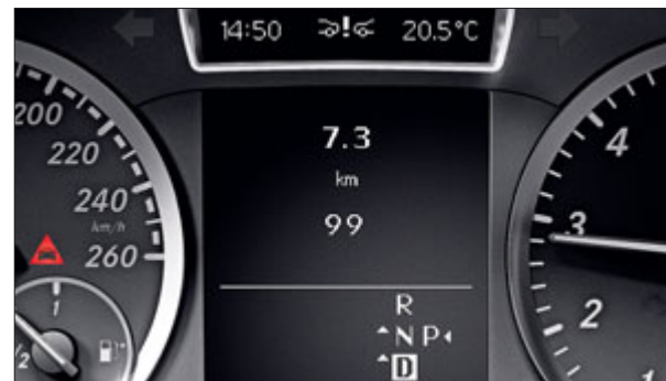
The COLLISION PREVENTION ASSIST can provide visual and acoustic warnings if the safety margin is too short
