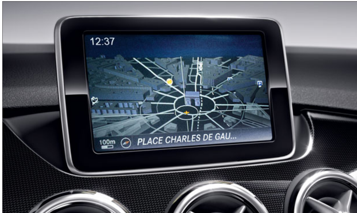
COMAND Online facilitates user-friendly operation of the main information and communication functions via a single, high-resolution colour display with a diagonal of 17.8 cm
