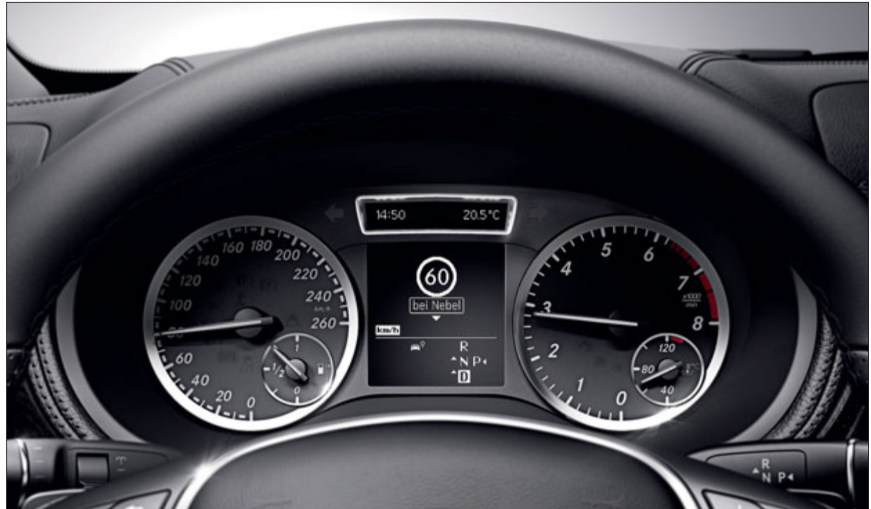
The Speed Limit Assist can remind the motorist about the speed limit currently in force
