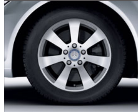
7-spoke light-alloy wheels with 195/60 R 16 tyres (standard for C 180 BlueEFFICIENCY, Code R20) or 205/55 R 16 tyres (standard for C 220 CDI BlueEFFICIENCY, Code R75)
