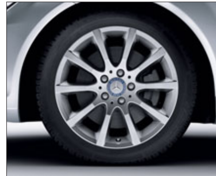
10-spoke light-alloy wheels with 225/45 R 17 tyres (standard for C 250 CDI BlueEFFICIENCY, C 250 BlueEFFICIENCY and C 350 BlueEFFICIENCY, Code 25R)
